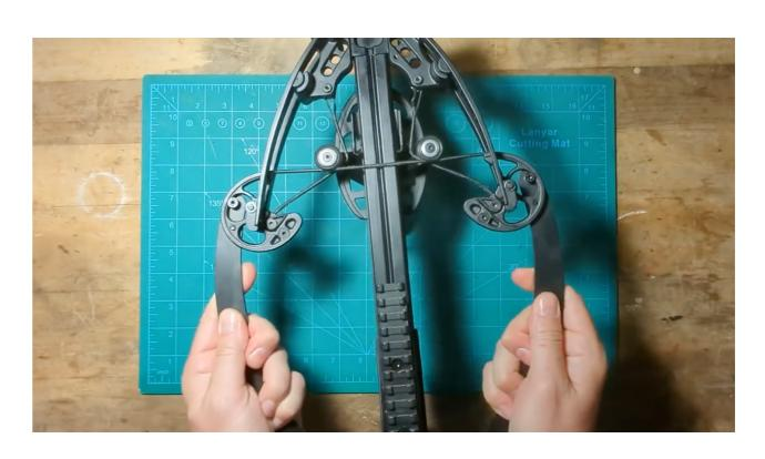
4. Unscrew the bolts that secure the cables to the cams.
