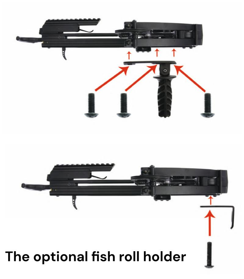
When attaching the fish roll holder, it is important to make sure that only the middle one of the three screws is loosened in order to tighten the fish roll holder. The two outer screws hold the bow unit in place and to avoid injuries, they must not be unscrewed.
