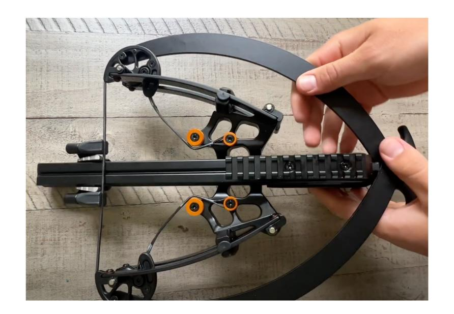
5. Fasten the press and attach the free ends of the cables to pulleys.
