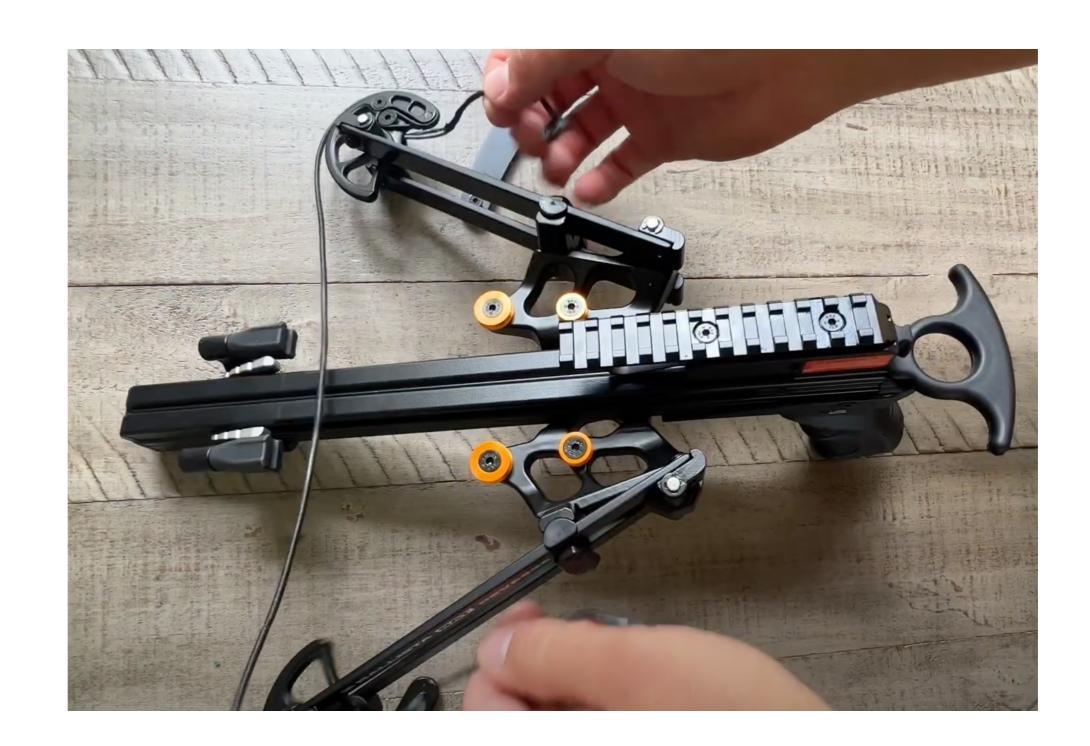
4. To replace the cables, unscrew the bolts that secure the cables to the cams.
