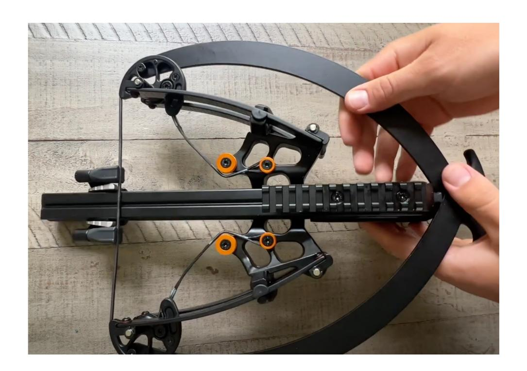
2. Remove the cables from the pulleys.
